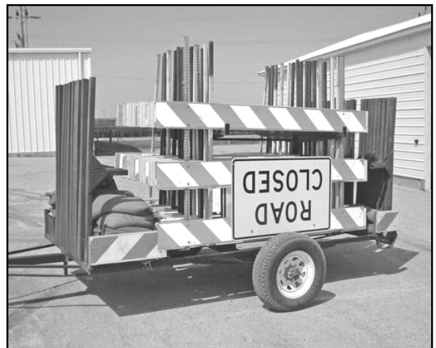
A sign trailer fabricated by Brookings County Highway Department which has Type III barricades and signs loaded and ready for quick response to emergency road closings.
