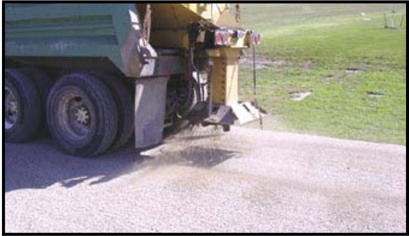
A "whirly bird" sander applies the necessary amount of sand in a uniform manner.
